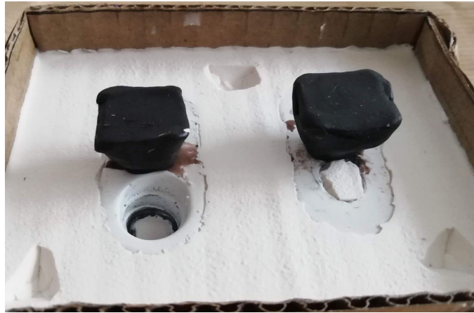
Figure 5. Ready to pour the second half of the rubber mold. Notice the wax sprue
