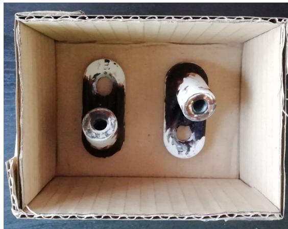
Figure 3. Two of the part prior to pouring the first half of the rubber mold
