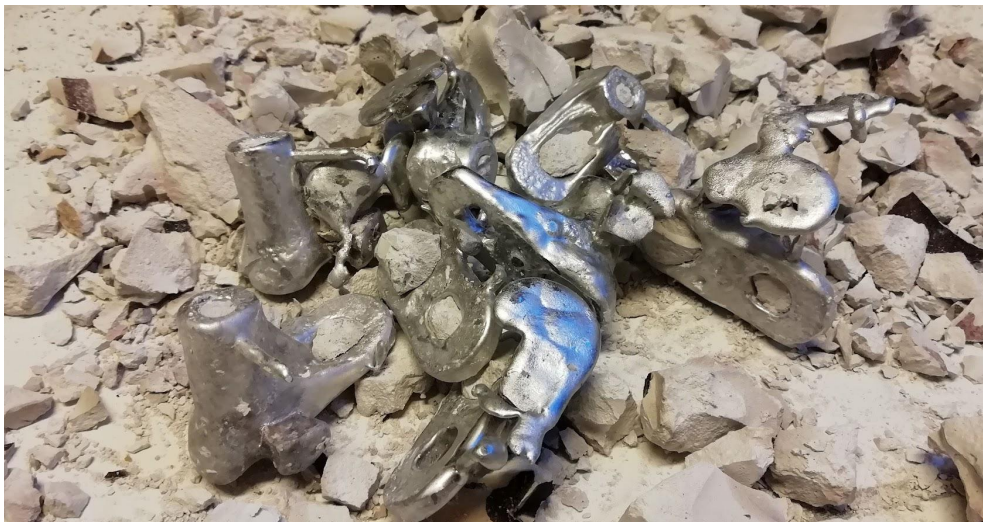
Figure 3. Metal parts and pieces of mold prior to cleaning
