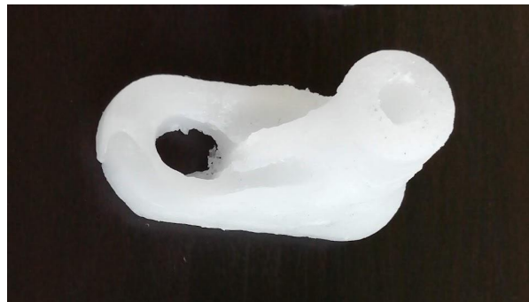
Figure 1. A wax copy of a chair brackets
