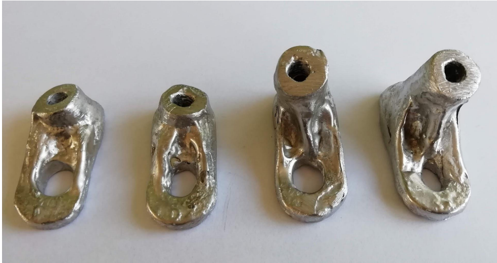
Figure 4. First batch of metal cast parts after cleaning
