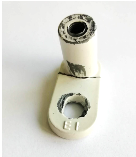
Figure 1. One of the failed chair brackets.
