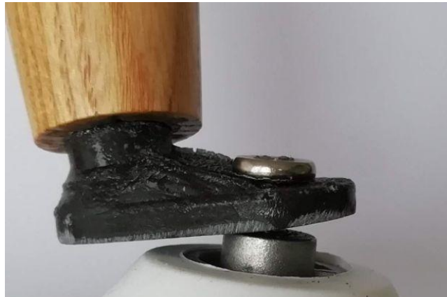
Figure 1. Polyester bracket installed (showing an angle mismatch (not the cause of failure))
