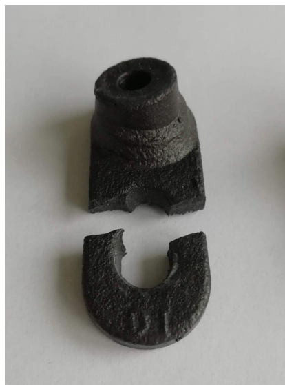
Figure 2. Failed polyester bracket
