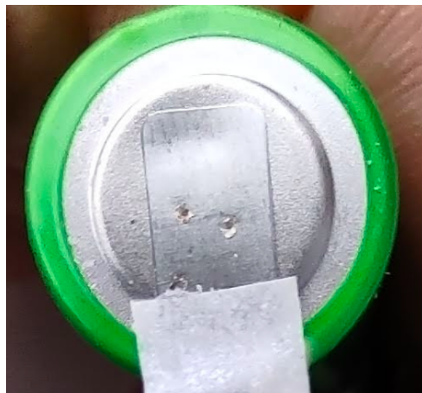
Photo 2 - Welded spot not centered on cell
